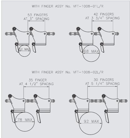
\*For diameter 93mm-96mm special pusher pad required
