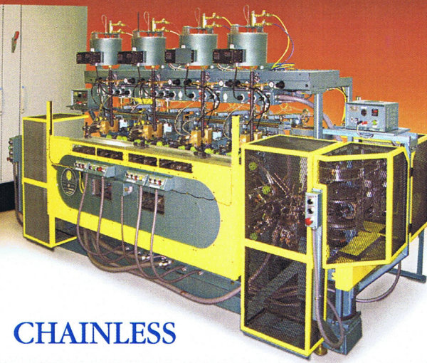
Optimum Production Body & Shoulder Decorating Machine
