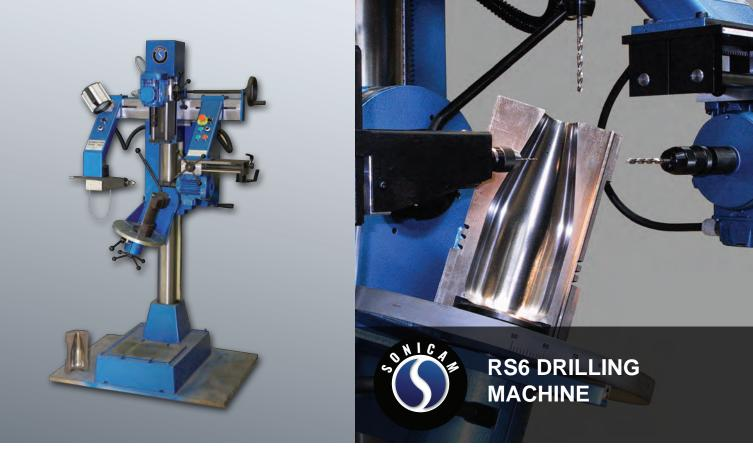
Sonicam RS6 is drilling tiny vacuum channels inside the moulds.
