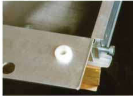
Having attached the Contact Bars, tension is applied with the side and end adjuster screws.
