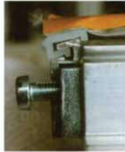
The special profiles lock together under tension to prevent loss of tension.
